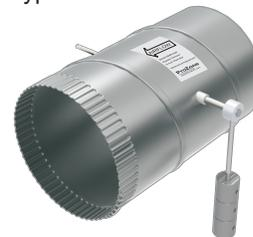
The bypass damper must be sized to bypass the total system CFM minus the CFM of the smallest zone. The weights on the arm of the bypass damper should be set so the damper is fully open and open enough to eliminate any noise that may occur when only the smallest zone damper is open.
