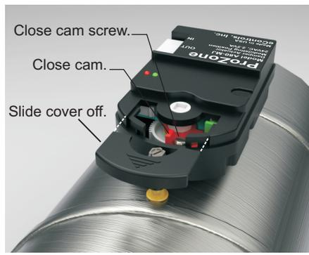
The slide off cover can be removed to adjust the close position from fully closed to about 50% closed. Loosen the screw holding the cam and rotate it clockwise and then tighten the screw.
