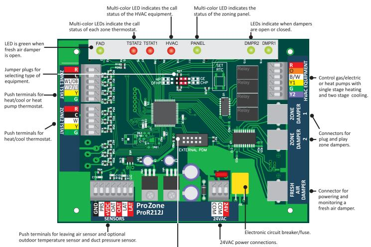
Connector for PDMi3 carried by installer to set options and clone multiple panels.
